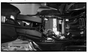
H- Attach the positive and negative wires to the battery.
