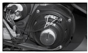
E- Use a T10 Torx driver to remove the rear pod speakers. Remove the speaker connections from the speakers. The wire harness will be used later in the install to connect to the stock wiring and speakers.
