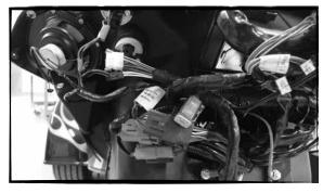
C- Keep track of which wires go to the clutch and brake side speakers.
