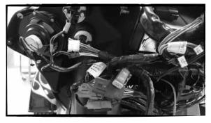
C- Keep track of which wires go to the clutch and brake side speakers.
