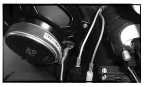
B- Connect the speaker output wires to the new speakers mounted to the bike. Also make sure to keep the clutch side and brake connectors directed to the correct side. The speaker output wires are marked with a tag indicating clutch or brake and have female fastons on each end that will connect to the new speaker.
