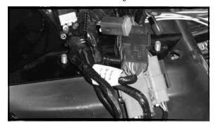
H- Place the amplifier bracket over these 2 bolts, and replace and tighten the nuts. The amplifier is now locked in place.(Amp pigtails face upward)
