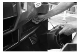
Step 8 - Reaching through the top of the dash, pull the wire up and through as you seat the pod in place in the dash.
