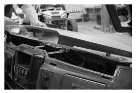
Step 4 - Prepare the speaker pod by removing the four (4) T20 screws holding the speaker in place.
