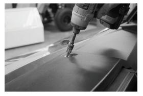
Step 2 - Remove the two (2) trim panel pin rivets found on either side of the dash cover.
