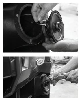
Step 11 - Install the speaker grilles using a the supplied Phillips head screws and a Phillips screwdriver or screw gun.
