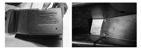
Step 7 - Start by feeding the speaker wire from the pod up into the dash area through the small holes located above the storage shelf on either side of the vehicle.
