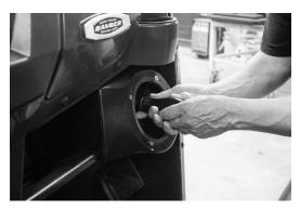
Step 10 - Reconnect the speaker to the speaker wires and mount the speaker to the pod using a T20 Torx driver and the screws removed in Step 4.
