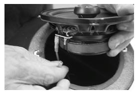
Step 6 - The speaker pods mount to the vehicle through the two (2) holes in the back of the enclosure through the back wall of the storage shelf using the provided hardware. Left and right pods are identified by ensuring the MTX logo on the back is right side up.
