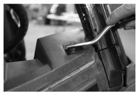
Step 3 - Lift and pull back the top dash cover to release the clips holding it in place.
