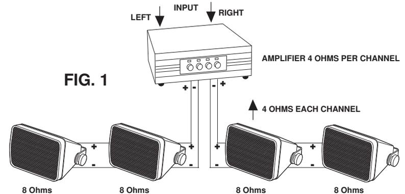
Be sure to use a good quality, unshielded twisted pair speaker cable to connect the amplifier to the speaker(s) (#14AWG for runs <80', #12AWG for runs >80'). Standard ZIP style speaker cable may also be used if twisted pair cable is not available.
