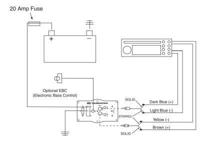
19. Plug power wire harness into amplifier pre-amp.
