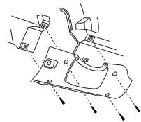
**14.** Remove (3) bolts holding the instrument cluster trim panel. Pull along edge to unsnap.
