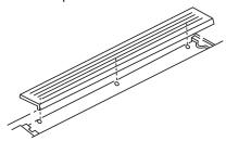
25. Using screws provided, install the enclosure into vehicle as shown below.
