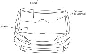
Note: To avoid any damage to parts inside engine compartment, drill from inside of vehicle using a short bit.
