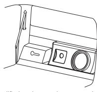
**2.** If externally amplified make speaker connections to the enclosure from the amplifier; loosen terminal knobs (a 13-mm nut driver can be used). Connect speaker wires from amplifier to enclosure, positive to red terminal knob and negative to black terminal knob. Refer to Step 25 for mounting directions.
