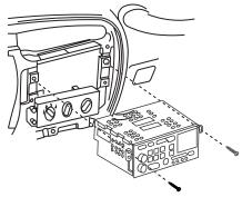
17. Behind the radio, locate the rear speaker wires. Colors are right channel; dark blue (positive) light blue (negative), and left channel; brown (positive), yellow (negative). Tap into wires with the supplied RCA High Level input wires and route over to driver's side threshold and to pre-amp of enclosure
